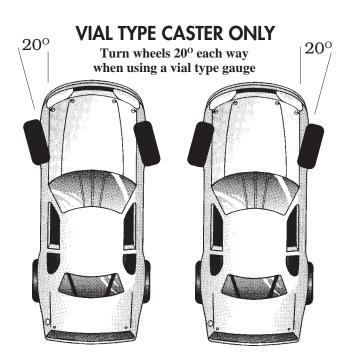
NOTE: Adjusting the caster may have an effect on the camber and vice versa. Double check all your settings before finishing. Be sure to tighten all suspension bolts when done.
