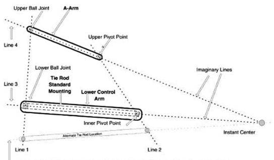
The outer tie rod end must intersect line 1. The inner tie rod end must intersect line 2 and the the tie rod angle must intersect with the instant center of lines 3 and 4.
