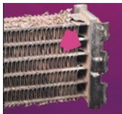
B. An electrochemical reaction that will produce voids in tubes.
