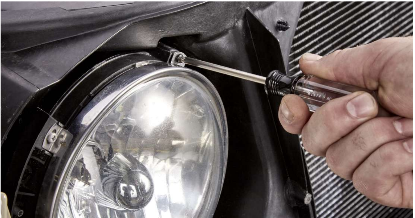
The headlamp bezel is held in place with 4 Torx screws. Note the parking lamp still attached.
