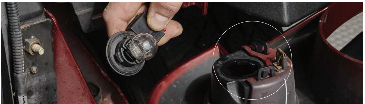
The parking light assembly has already been removed from its location in the grille (circled)
