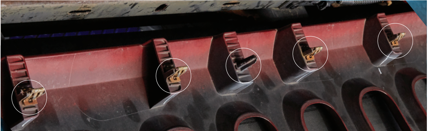
The bottom clips (circled) are disengaged by pulling at the bottom of the grille
