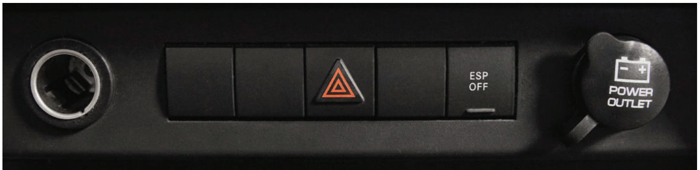
In our 2007 Wrangler, the LEFT 12 socket is hot only with key on, so this is one we used. The RIGHT socket is hot at all times.
