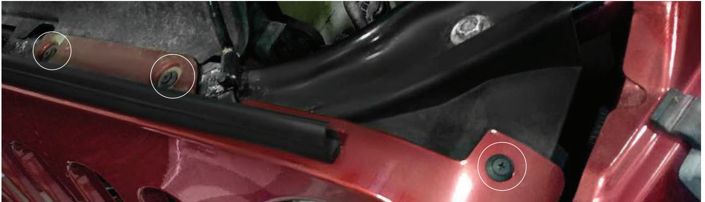
Circled are 3 of the clips to be taken out when removing the Jeep grille
