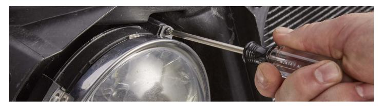
b. As the last screw is removed, hold onto the headlamp, as it could fall.
