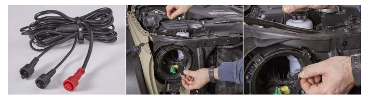
B Take one headlamp plug-n-play connector harness from the kit, and plug it into the factory harness. Be sure to secure the connection so the plug will not disconnect. A cable tie or electrical tape may be necessary if your slide lock does not "click".
