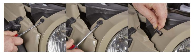
® Gently pull the top of the grille outward, away from the car. Reach down and release the parking lamp bulbs and holders, by turning them a quarter-turn. Keep them attached to the wire harness, and place them where they will not be damaged. (They can be left to hang in the opening between the bumper and the body of the Jeep.)
