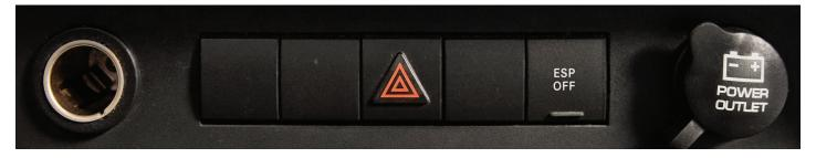
In our 2007 Wrangler, the LEFT 12V socket is hot only with key on, so this is the one we used. The RIGHT socket is hot at all times.
