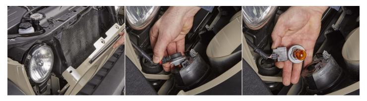
© The bottom of the grille is held in place by clips. Gently pull on the bottom of the grille until the clips disengage; remove the grille from the car and put aside in a safe place.
