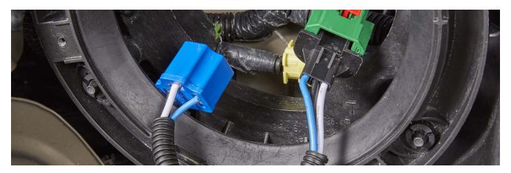
© Connect the corresponding wires from the headlight assembly to the new wire and harness. Now, repeat on the other side of the vehicle.
