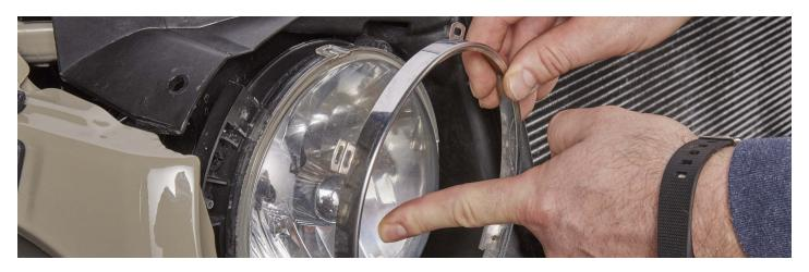
c. Remove the bulb from the assembly with a ¼ turn, remove the headlamp assembly from the car and put it in a safe place. Unplug the factory harness from the bulb, this may involve unlocking the red slide lock.
