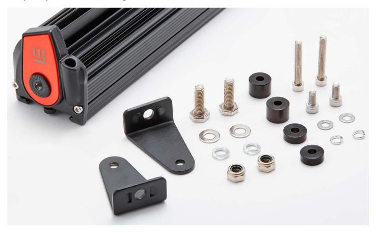
If no spacers are necessary, attach the brackets to each side of the light bar using the 5mm hex wrench, small bolts and washers. Bracket orientation can be changed based on preference.
