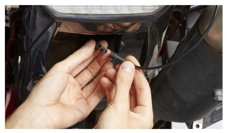
**STEP 6.** Run the wires from the base to the battery. Make sure the harness does not come into contact with any hot exhaust components or suspension parts. Use cable ties to secure the harness to the vehicle.
