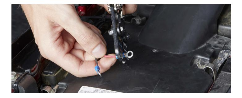
**STEP 9.** Connect the ring terminals to the battery terminals.
