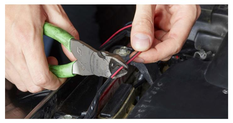
**STEP 8.** Strip the wires, then connect the ring terminals to the ends of the wire.
