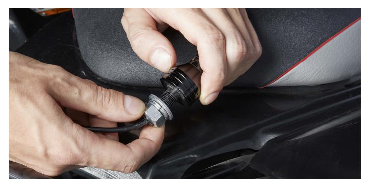
**STEP 4.** First slide the wire through the attachment location, then place the threaded end of the base through the attachment location. Slide the flat washer onto the threaded end of the base, slide the lock washer on after the flat washer, then screw the nut onto the bottom of the base. Tighten the nut with a 19mm wrench.
