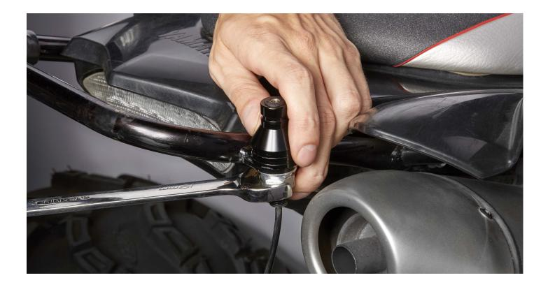
**STEP 5.** Connect the base to the wiring harness by lining up the arrows and tightening the lock on the connector.
