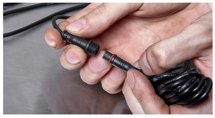
**STEP 16.** Plug in the RGB wires to the wires coming out of the LED controller.
