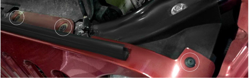
Circled are 3 of the clips to be taken out when removing the Jeep grille
