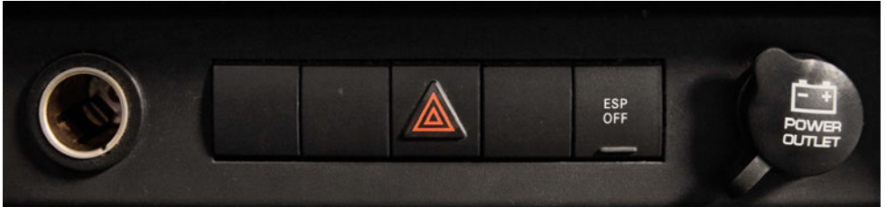
In our 2007 Wrangler, the LEFT 12 socket is hot only with key on, so this is one we used. The RIGHT socket is hot at all times
