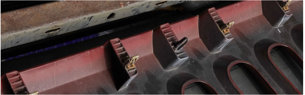
The bottom clips are disengaged by pulling at the bottom of the grille
