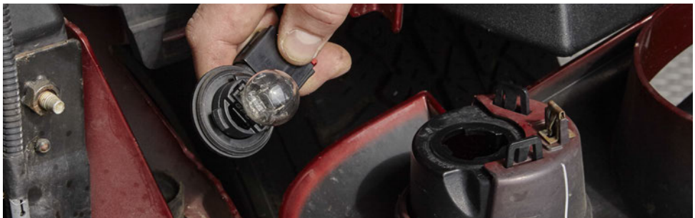
The parking light assembly has already been removed from its location in the grille
