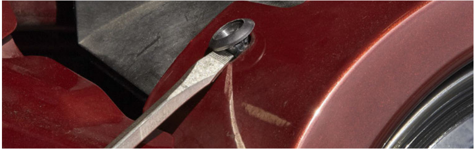
Use pliers and/or flat blade screwdrivers to remove clips (clip design may be differ on your vehicle)
