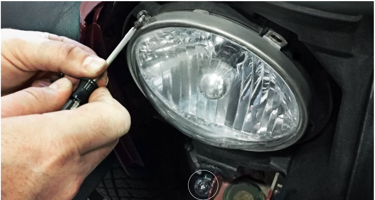
The headlamp bezel is held in place with 4 Torx screws. Note the parking lamp still attached (circled)
