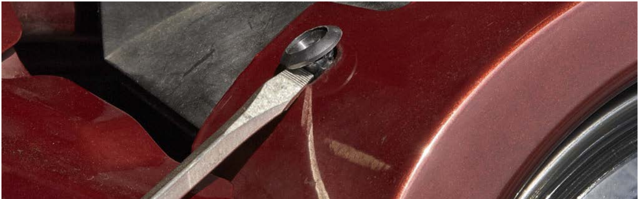
Use philips and/or flat blade screwdrivers to remove clips (clip design may be differ on your vehicle)
