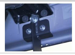
Locate the middle mounting location and one of the universal mounting brackets.
