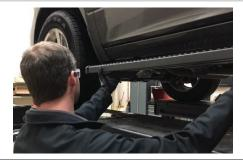
Repeat steps 8 through 11 to install the running board to the brackets on the passenger side of the vehicle.
