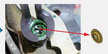
2.Remove/Install the spring washer smooth.
