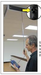
Probe will measure dry bulb, wet bulb, relative humidity, dew point, air velocity and air volume.
