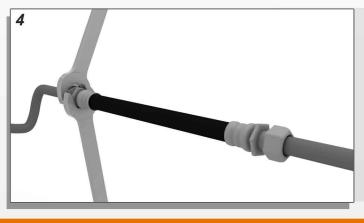
With the steel lines clean and deburred, put a small amount of oil on the end of the line before sliding the repair line fitting over the steel line. The fittings are shipped assembled but loose so it will bottom out in the fitting. Tighten the nut on the repair line fitting until you can no longer turn the steel line in the fitting. After lining up the orientation of the line as noted in step 2, you can tighten the other side.
