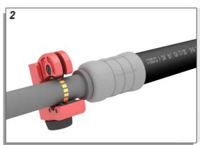
Layout the line so as to note the orientation of the bends to aid in reassemble. Using a mini pipe cutter, cut the steel line as close to the crimp as possible, removing the crimped rubber line.
