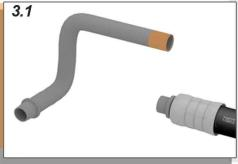
The cut ends of the steel line need to be deburred before installing the repair kit. A piece of scotch bright or emery paper works well for this, as well as removing any light surface debris.
