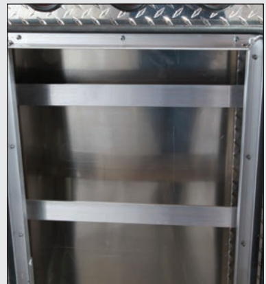
Chain hangers in each side compartment
