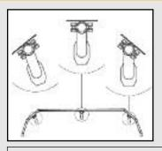
All three E - Z fender brackets are adjustable in length from 27" to 30".
