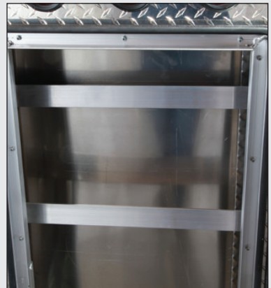
Chain hangers in each side compartment
