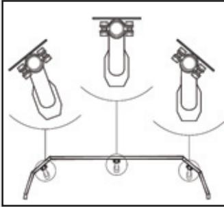
All three E - Z fender brackets are adjustable in length from 27" to 30".
