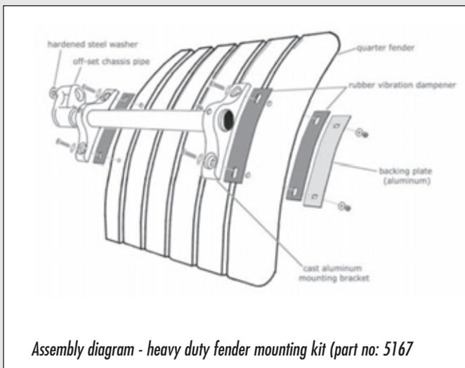
Assembly diagram - heavy duty fender mounting kit (part no: 5167)
