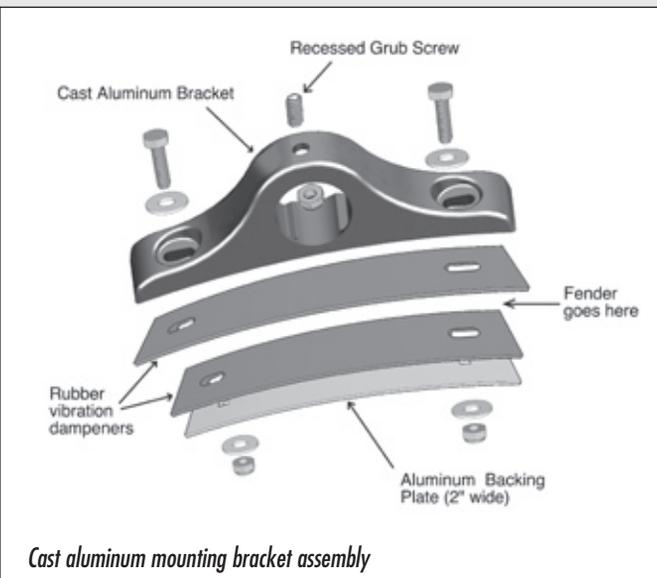
Cast aluminum mounting bracket assembly
