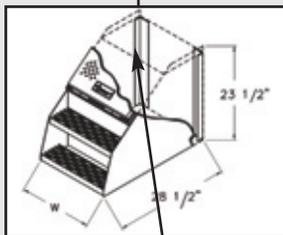
24", 30" and 36" saddle boxes are reinforced with side gussets to accommodate larger loads.
