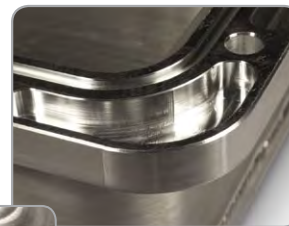
O-ring groove in fully machined pan rail
