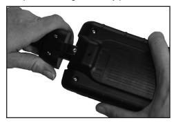
4. To attach a new cable, align the cable and tester housings and push together. Insert the screw and tighten.
