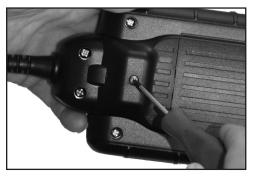
3. Grasp the housing and firmly pull the cable assembly from housing.
