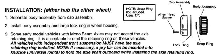
4. Place cap assembly on body assembly and secure with six socket head cap screws. Torque to 27-31 in. -lb. (31-35 kg. cm.).
