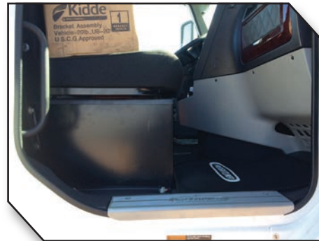
Figure 6 - Passenger Seat with Under Seat Battery Storage
