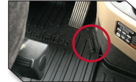
Figure 11 - Driver Mat Hook Installation
