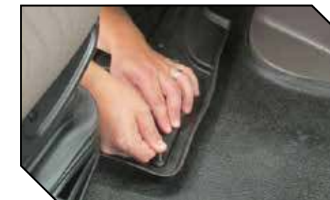
Figure 14 - Apply Pressure to Hook
