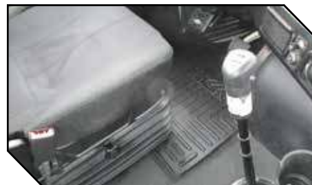
Figure 13 - Driver Mat Hook in Position
