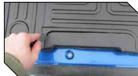
Figure 11 - Hand Trimming for Seat with Rubber Boot
