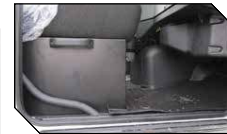
Figure 17 - Fixed Base Passenger Seat with Trimmed Mat
