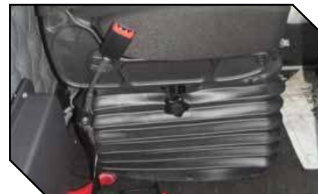
Figure 11 - Hand Trimming for Seat with Rubber Boot
