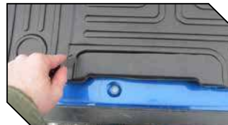
Figure 11 - Hand Trimming for Seat with Rubber Boot
