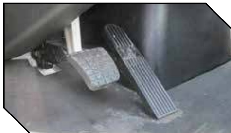
Figure 2 - Floor Mounted Throttle Pedal Mechanism
