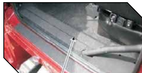
Figure 6 - Driver Side Electrical Tray
