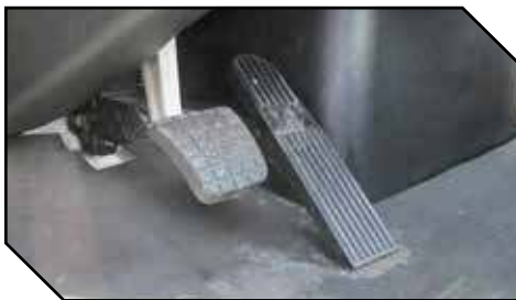
Figure 2 - Floor Mounted Throttle Pedal Mechanism
