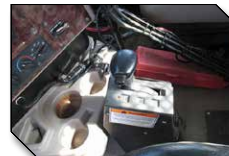
Figure 8 - Floor Mounted Control Tower
