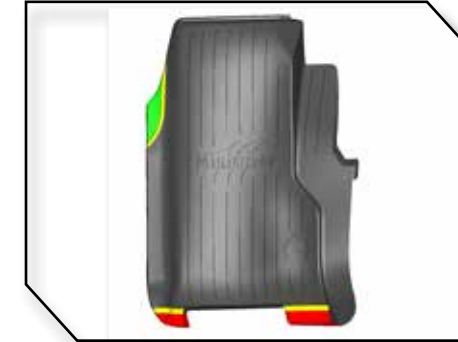
Figure 9 - Passenger Mat Trimming Diagram
