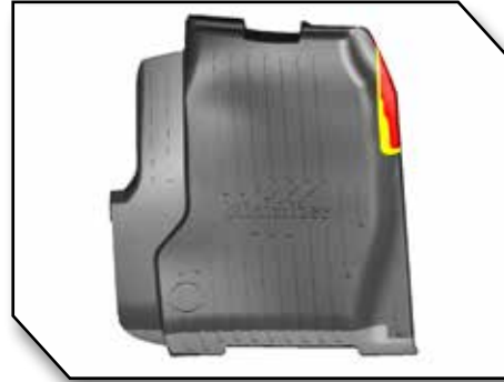
Figure 5 - Driver Mat Trimming Diagram
