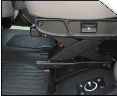
Figure 1 - National Driver Seat with Suspension Base
