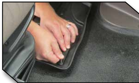
Figure 7 - Apply Pressure to Hook
