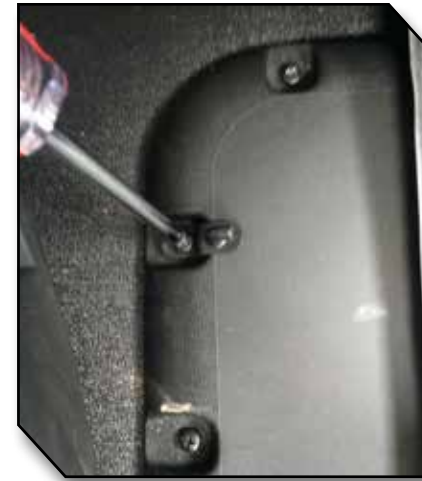
Figure 7 - Retention Hook Installation
