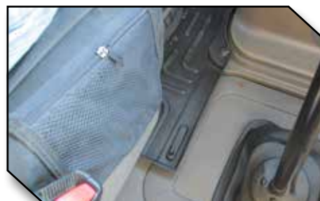
Figure 10 - Driver Mat Hook Installation
