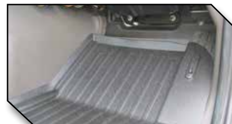
Figure 12 - Properly Installed Driver Mat and Hook
