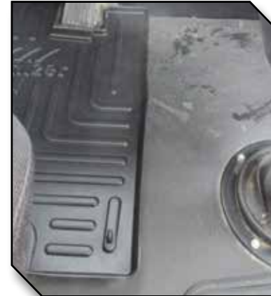
Figure 9 - Driver Mat Hook Installation
