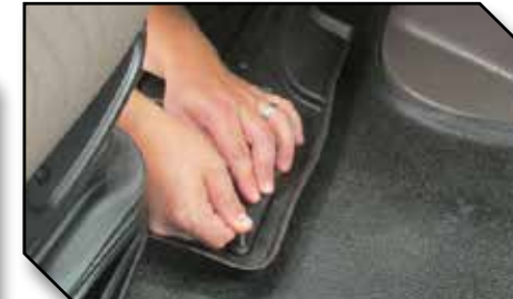
Figure 10 - Apply Pressure to Hook
