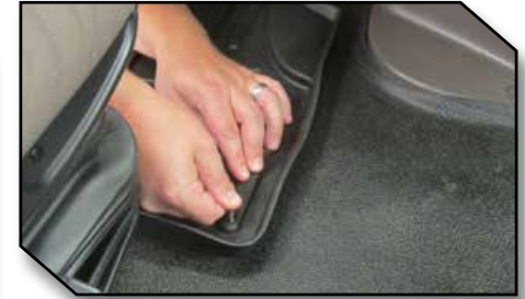
Figure 7 - Apply Pressure to Hook
