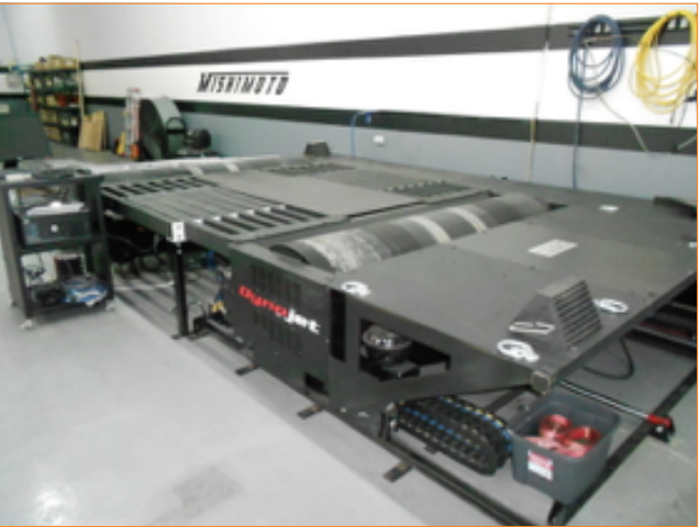
FIGURE 3: A Dynojet™ dynamometer was used for vehicle testing.
