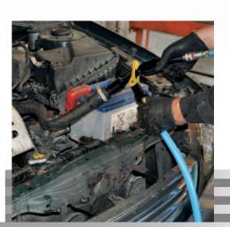
Includes Spray Washer MV4570 Cooling System Flusher
