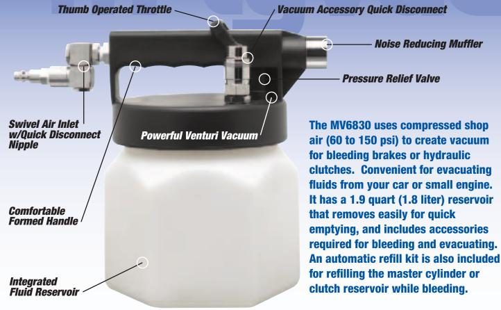
The MV6830 uses compressed shop air (60 to 150 psi) to create vacuum for bleeding brakes or hydraulic clutches. Convenient for evacuating fluids from your car or small engine. It has a 1.9 quart (1.8 liter) reservoir that removes easily for quick emptying, and includes accessories required for bleeding and evacuating.
