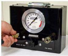
Step 1 Couple shop air to input side of tester. (Minimum of 80lbs. PSI / Max of 100lbs. PSI.)
