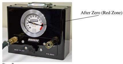
Step 2 If needle reads after zero (Off Scale In Red Zone) continue to step 3. If the needle reads before zero (100-0 Range) continue to step 5.
