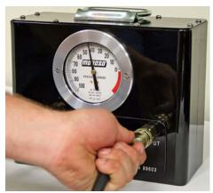
Step 4 Insert whip line until air is heard purging from system, <u>disconnect whip line</u>, the needle should now be in the 100-0 range. Continue to step 5. <u>NOTE</u>: If needle is not in this range repeat step 3. (Goal is to get needle in 100-0 range)
