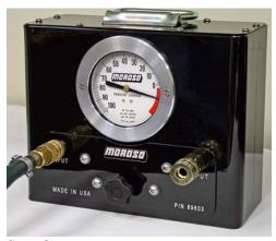
Step 3 Turn adjuster counter clockwise approx. 2-3 turns. Needle will not change position drastically until air is purged from system in step 4.
