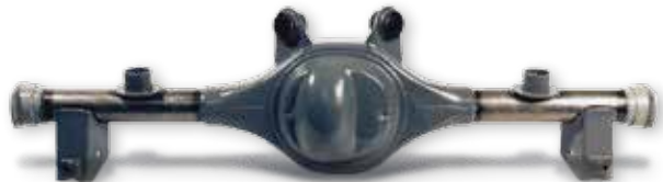
9" Bolt-In Housing - GM G-Body 1978-87 Grand National, Cutlass, GTO, Grand Prix, Chevelle 9" Bolt-In Housing & Axle Package - GM G-Body
