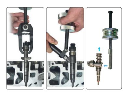
**Universal kit for diesel injectors.** Fits Bosch, Delphi, Denso, and Siemens. Will work in most cases without removing the electric plug.
