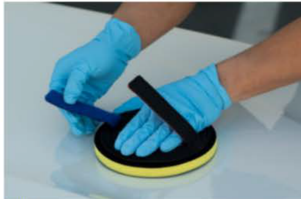
Step 3: Place fingers in a comfortable position in hand strap.
