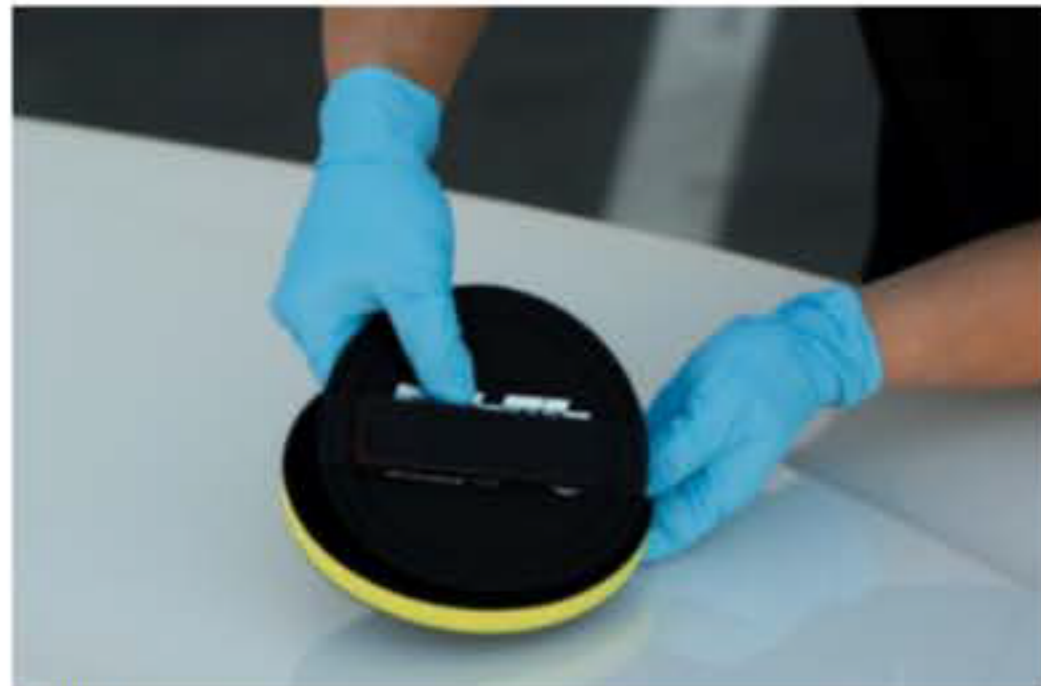
Step 1: Center and attach the hand strap to the back of the Autoscrub pad
