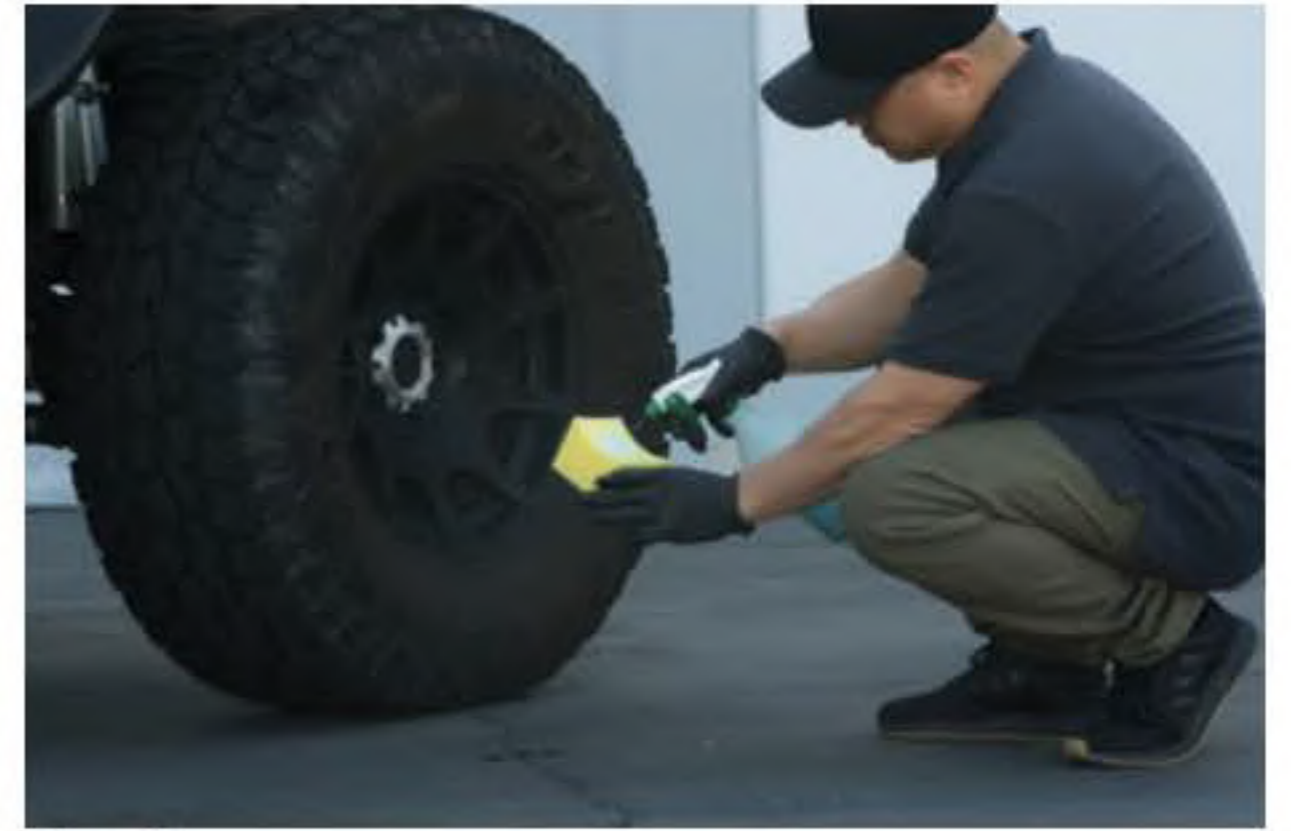
Step 3: Spray a generous amount of mixed Blue Dress onto applicator pad.
