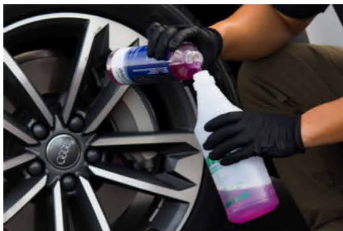
Step 1: Mix concentrated Non Acid into sprayer bottle using 4:1 mix ratio with water
