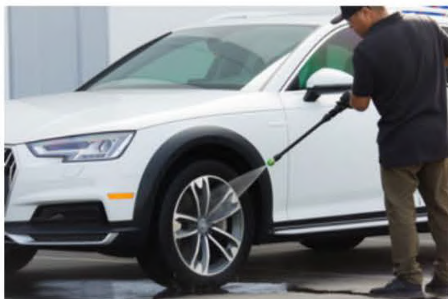
Step 6: Rinse wheels and tires with water. Preferably a power sprayer for non touch removal and cleaning
