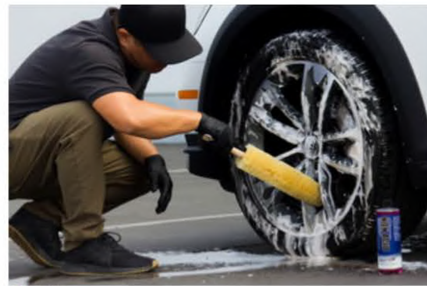
Step 5: Allow Non Acid to dwell on tires from 1-3 minutes. Agitate Non Acid if necessary with wheel brush. *do not let Non Acid dry on wheels
