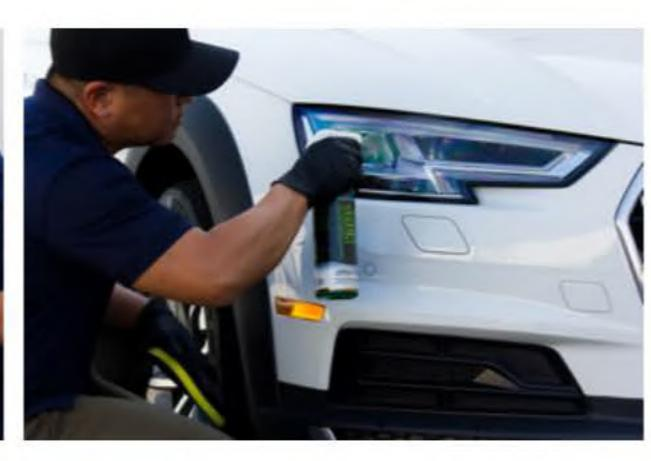
Spray sufficient amount of lubricant on the plastic surface. NOTE: Do not allow the lubricant to run dry on the surface.
