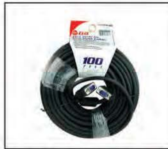
VGA-M-M-100 VGA MALE TO VGA MALE CABLE • Ideal for high resolution monitors (1024x768 and above) • Triple-coaxial + twisted-pair wire for crystal clear images • Impedance matched @75 ohms for full brightness and vibrant pictures color • Ferrite core eliminates EMI interference • Molded connector ends with strain relief • 100'
