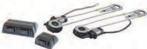
PROW-2002 UNIVERSAL POWER WINDOWS • with 3 switches (2 window power window kit) • Complete kit to convert 2 manual windows to full power • Power window system • Installed behind the door panel • Cuprum bearing • POM plastic gear wheel
