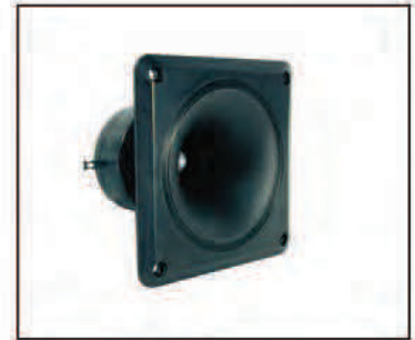
NTX-4545PZ 4.5" X 4.5" TWEETER • Frequency Range: 2K~20KHz • Power RMS/Max: 75/150W • Impedance: 4-8 Ohm • Mounting Diameter: 85mm
