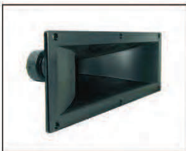
NTX-1405PZ 15-1/4" X 5" WIDE DISPERSION PLASTIC HORN • Frequency Range: 3.5K~20KHz • Power RMS/Max: 75/150W • Impedance: 4-8 Ohm • Mounting Diameter: 347mm x 96mm
