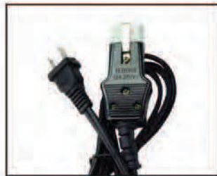
CMC-200 APPLIANCE ELECTRICAL CORD • Connector made of ABS and Bakelite for resistance to extreme heat. • Cable: 2*38*0.14 CCA • OD: 3.8*7.6 • 10A 250V • 6FT
