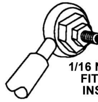
Figure 8 Schematic of "Drilled Out" Banjo Fitting
