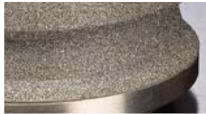
CLOSE-UP OF REVERSE-PLATED DIAMOND FORM ROLL
