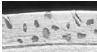
MICROSCOPIC VIEW OF A CONVENTIONAL INFILTRATED CNC DRESSING DISC EDGE
