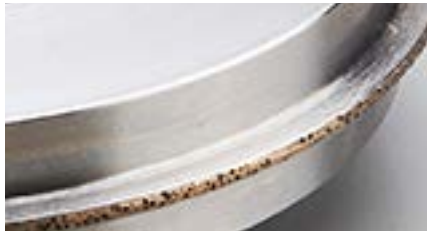
CLOSE-UP OF IDW DRESSING DISC DIAMOND EDGE
