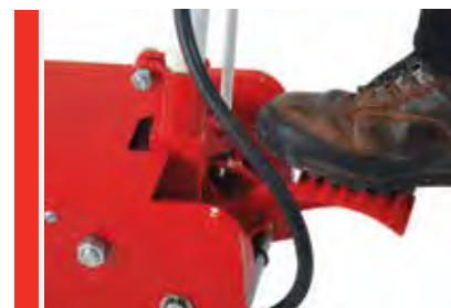
Foot pump for a fast lift to lift point*
