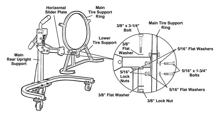
4. Secure the main tire support ring / lower tire support assembly to the horizontal slider plate using a 3/8" x 3-1/4" bolt, two 3/8" flat washers, and a 3/8" lock nut.
