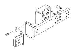
Mount No. 60581 to the starter side of the engine **with** No. 51400 end adapter in place.
