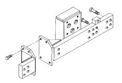
Mount No. 60581 to the starter side of the engine **with** No. 51400 end adapter in place.
